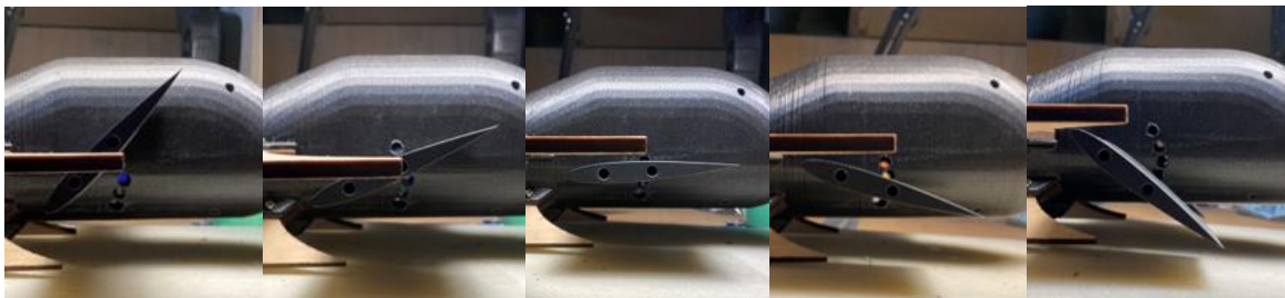
Figure 8: NACA 0012 Hydrofoil at Discrete Angles, (Left to Right: 45^\circ , 18^\circ , 0^\circ , -18^\circ , & -45^\circ ), BlueFry II.
