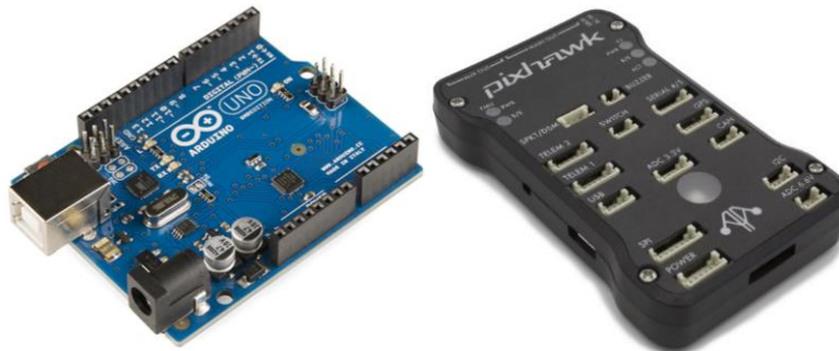
Figure 36: Arduino UNO MCU [13] (Left) and Pixhawk Flight Controller [14] (Right).
