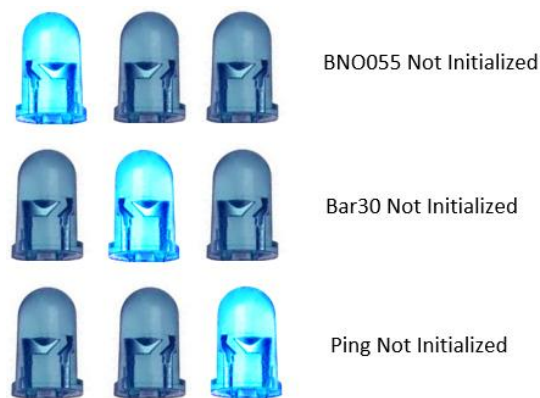
Figure 45. LED Indication of Sensor Initialization.
