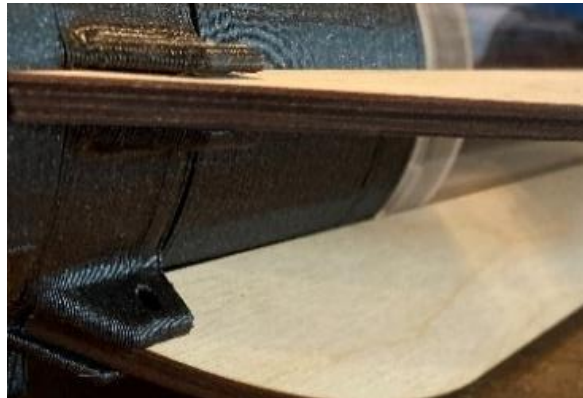
Figure 24: Original Static Fins and Keel Mounting Feature, BlueFry I and II.
