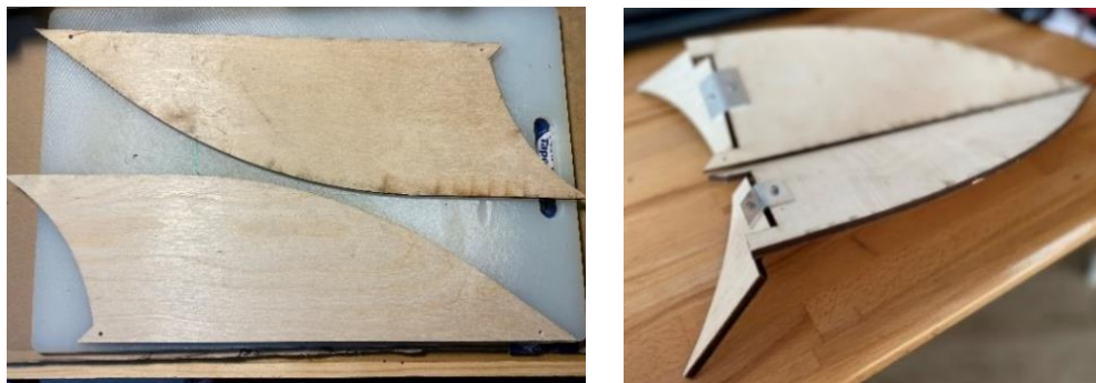
Figure 4: Static Fins (Left) and “Dynamic” Control Surfaces [Modified Static Fins] with 45^\circ Foils (Right), BlueFry I and II.
