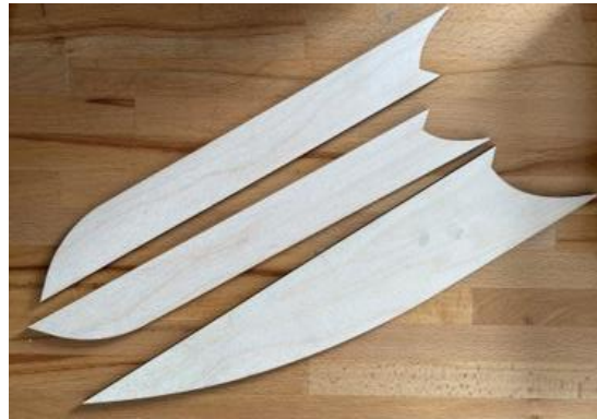
Figure 5: Full Keel (Bottom) and Bilge Keel (Top), Laser Cut Keels, BlueFry I and II.
